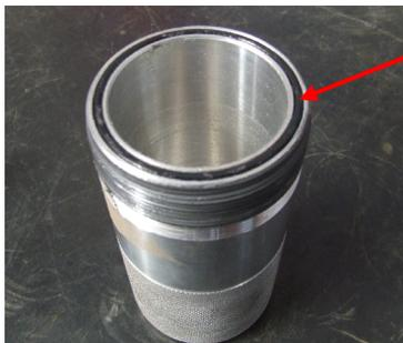
Fit the new head to bowl O ring seal (supplied) to the bowl in the position shown.
