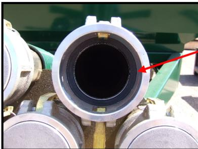
Finally, before reconnecting the primary hoses, make sure that there is a sealing ring in the female section of the camlock as shown.
