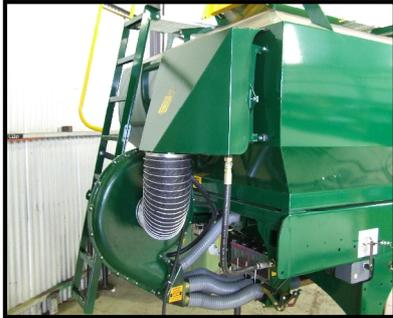
The oil cooler is protected by a relief valve which is pressure set in the factory to divert oil in the case of a pressure build up. A pressure build up is commonly caused by a restriction in the hydraulic return line usually being a quick release coupling being uncoupled.
