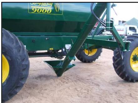
To place auger in an unload position, manoeuvre the auger and the arms so that the hopper can be placed under a bin clean out door.
