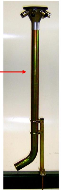
The metered product, once transferred to the secondary head, with the assistance of air volume and gravity flows out through the outlets to the sowing boots via the terminal lines.
