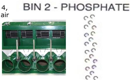
Metering Unit vanes positioned to mix 'N' FERTILISER with 'P' FERTILISER in Lines 1 & 3
