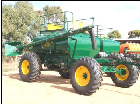
Load/Unload auger in the stowed position
