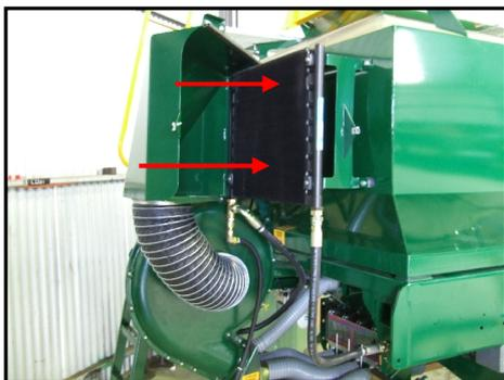
The hydraulic oil cooler fitted to all Simplicity Airseeders should be periodically checked and cleared of trash build up.
